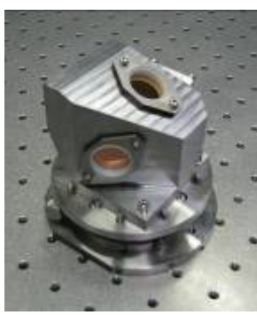
Manufactured RISTRA cavity with mounted cavity mirrors.
