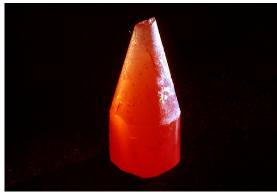
Fig. 1. As-grown LGiSe boule.
